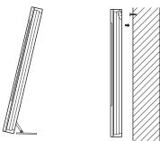
To have the indoor weather station free standing, simply unfold the stands on the back and set on a stable flat surface
